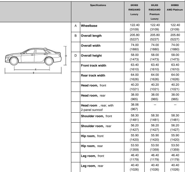
Published dimensions indicated are without optional equipment or accessories. Additional accessories or equipment ordered at the customer's request can result in a minor change in these dimensions.
